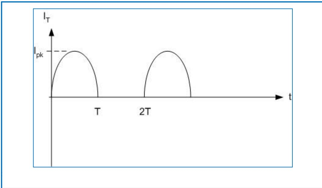
Fig. 1. Half wave conduction – e.g. an SCR at full power on AC mains.
