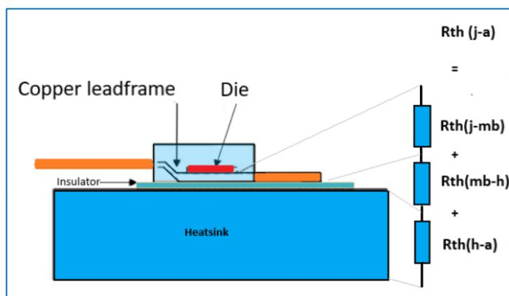
Fig. 3. Composition of thermal resistance for the TO220 package
